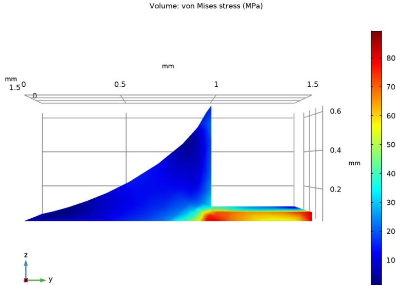
*Figure 5: Close-up of the von Mises effective stresses in the solder joints.*
