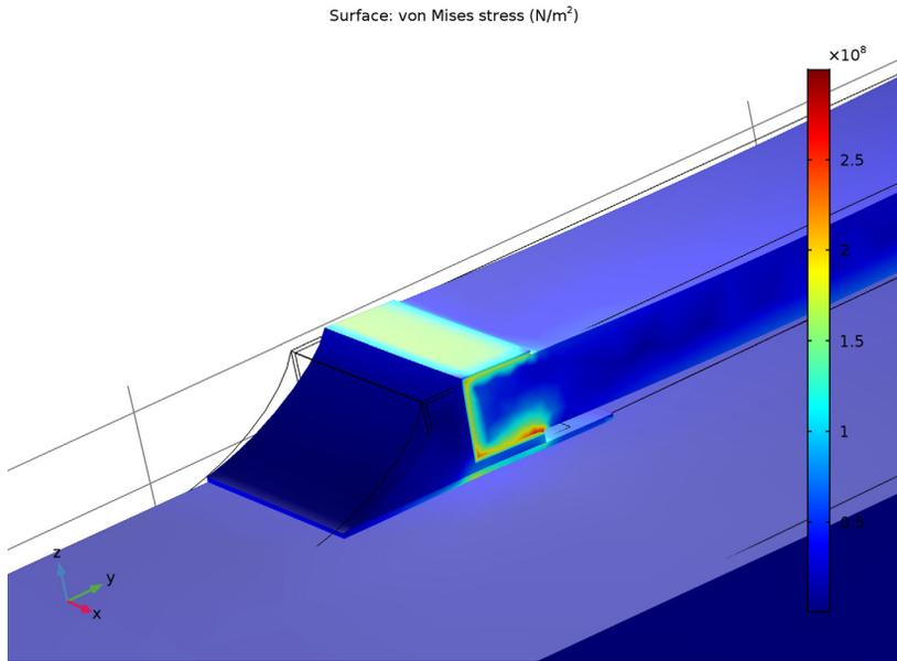
*Figure 4: The thermally induced distribution of von Mises effective stress together with the deformation (magnified).*
