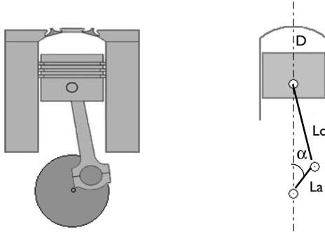
*Figure 1: The volume of a combustion cylinder can be expressed as a function of time with the slider-crank relationship. The diagram shows the key geometric parameters.  $L_a$  is the length of the crank arm,  $L_c$  is the length of the connecting rod,  $D$  equals the cylinder diameter, and  $\alpha$  is the crank angle.*
