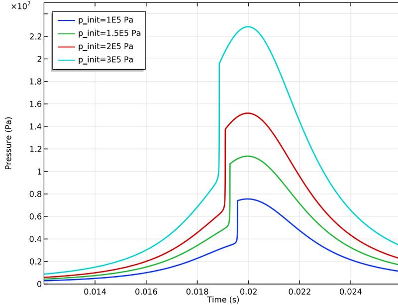
Figure 4: Increased initial gas pressure advances ignition times.
