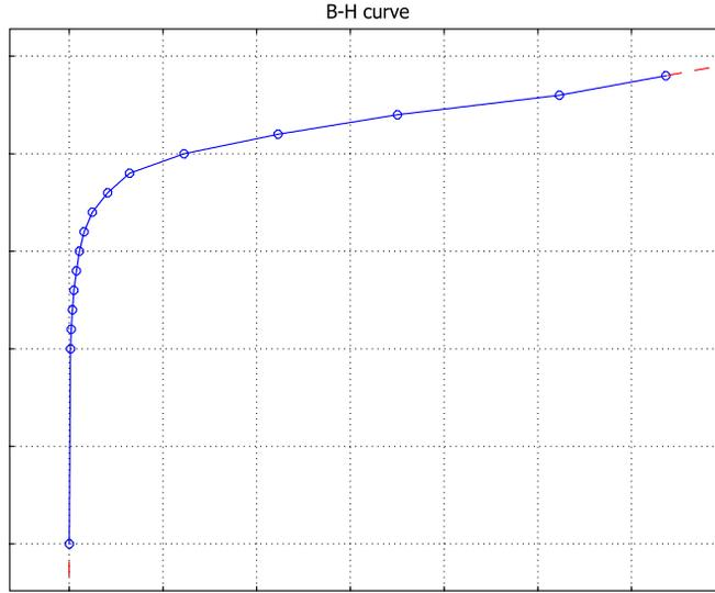
Figure 2: The norm of the magnetic flux,  $|\mathbf{B}|$ , versus the norm of the magnetic field,  $|\mathbf{H}|$ , for the rotor and stator materials. The inverse of this curve is used in the calculation.
