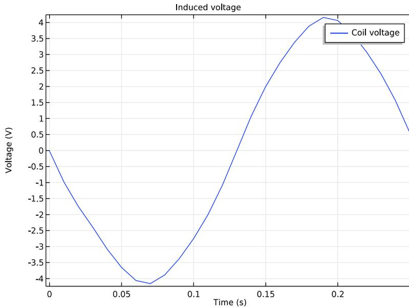
The plot shows an induced EMF with an amplitude of about 4.2 V
