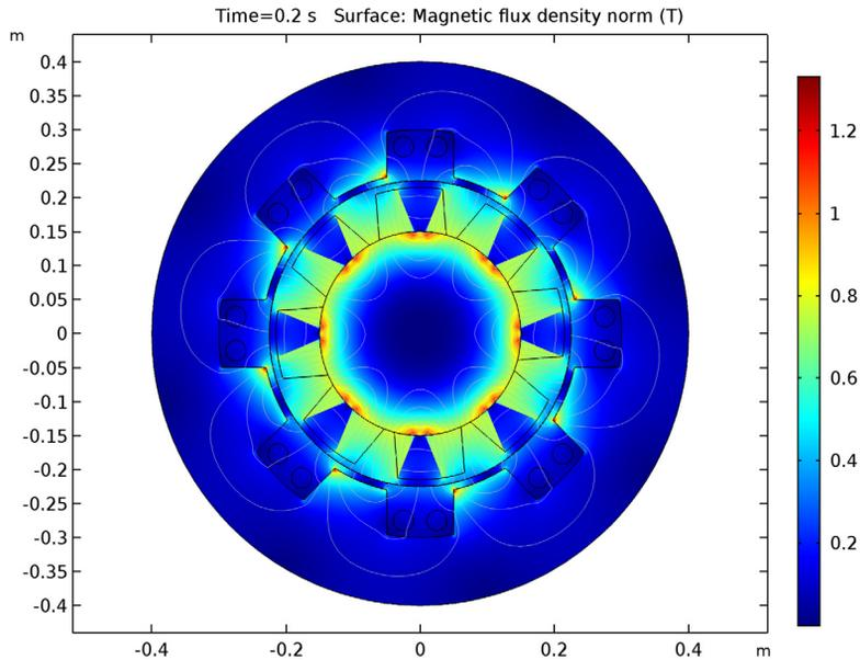
The plot will show the rotor position at  $t = 0.2$  s, the magnetic flux density norm and magnetic flux lines. Next, plot the induced EMF in a quarter of the cycle.
